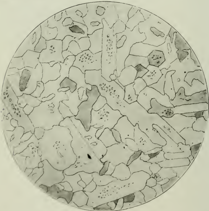
FIG. 20.—Silicified limestone ("Jaspeorid"), Aspen, Colorado, Cross Nicols. All quartz. Small inclusions of calcite in some of the grains. Magnified 30 diameters. (After Lindgren, T.A.I.M.E., Vol. XXX, p. 628). This shows the process completed. Complete outlines of earlier formed, automorphic crystals are seen in the later replacement silica, which is xenomorphic.
